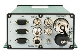
The LD5 Integrated Mobile Unit data ports.
