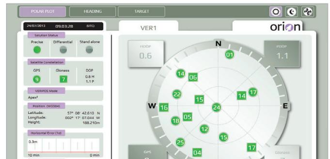
The above image is a display of a GNSS polar plot and position status information in Orion Software.
